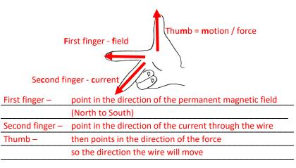
Annotate the diagram and explain the directions of the forces on the wire and the magnet and compare their sizes.
