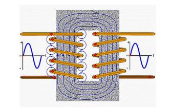
The coil of the circuit in the primary coil is carrying an alternating current, which produces an alternating magnetic field.
