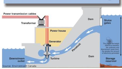
Describe the changes involved in the way energy is stored in the system above. Starting at the Sluice Gates on the right. Include the energy stores and transfers at each stage.
