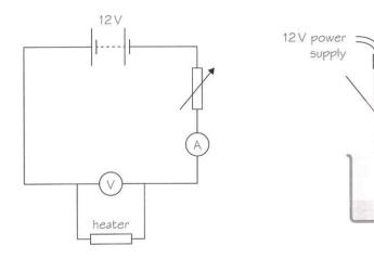
The student sets the current to  $4.0\,\mathrm{A}$  and the potential difference across the heater to  $8.0\,\mathrm{V}$  using the variable resistor. She runs the experiment for exactly 5 minutes.
