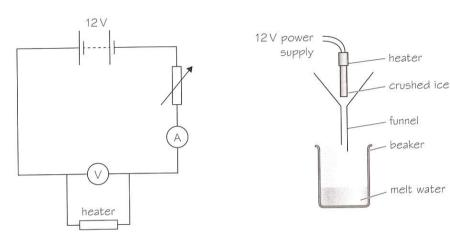
The student sets the current to 4.0A and the potential difference across the heater to 8.0V using the variable resistor. She runs the experiment for exactly 5 minutes.
