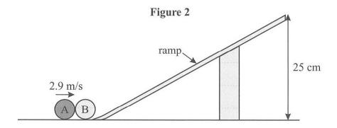
Before the collision, Marble A travels with a speed of 2.9 m/s and Marble B is stationary. After the collision, Marble B travels fast enough to just reach the top of the ramp, 25 cm above the ground.
